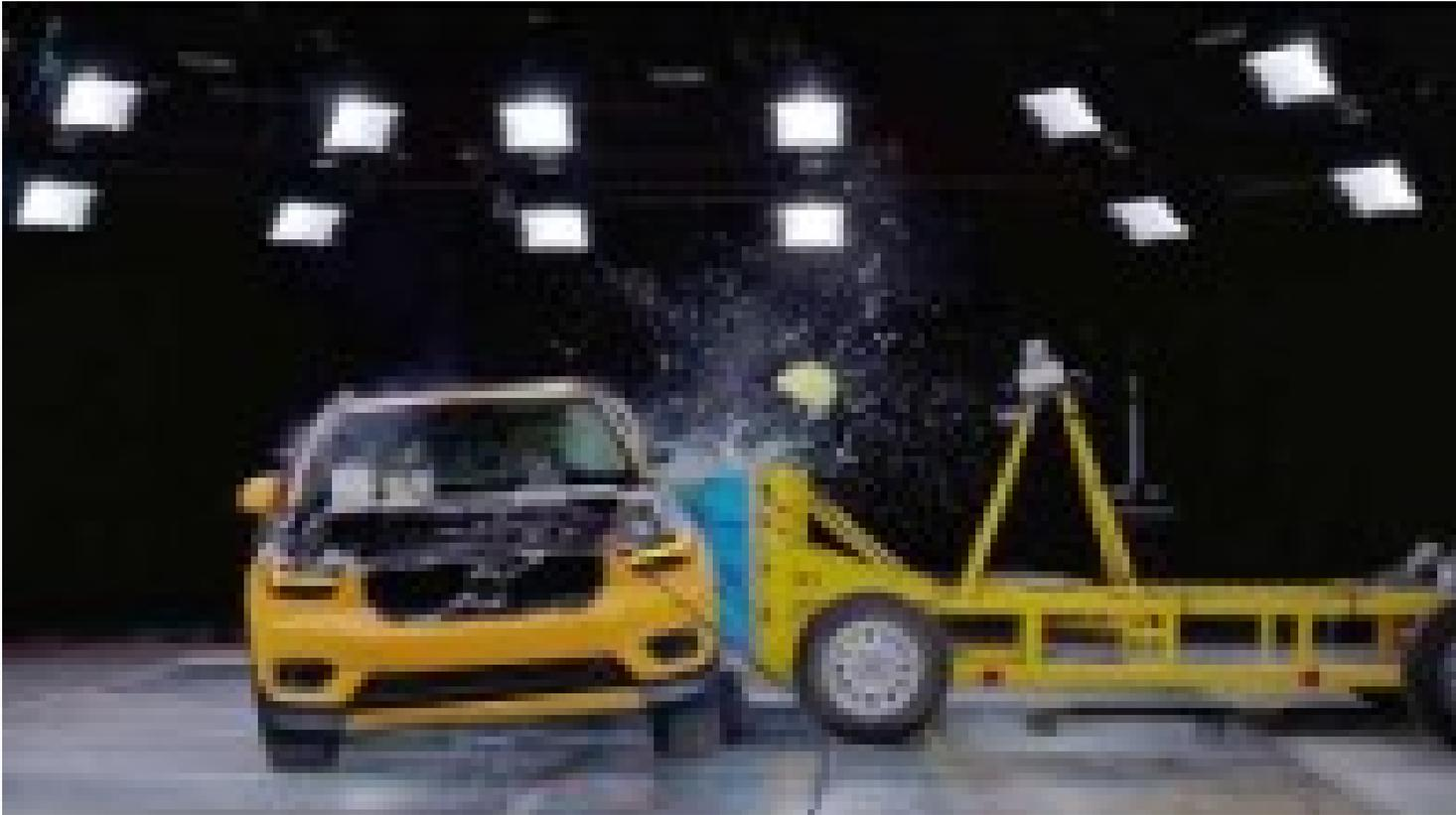
50 km/h, 950kg trolley. Test vehicle at “kerb weight” + 100kg
